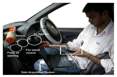
Figure.1 Photographic image of Experimental set up
