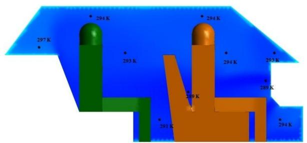
Figure.4 Temperature distributions for human load of 4
